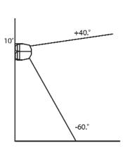
Standard speakers require a mounting bracket to accurately direct sound. The computer-aided design of the 13350 and 13351 provides optimal sound coverage, eliminating the need for mounting hardware and brackets. All wiring is terminated within the weatherproof speaker housing, again removing the need for installing costly junction boxes.
